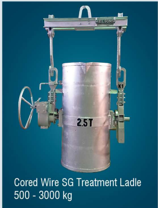
SG Treatment cum Pouring Ladle 300 Kg - 2 Mt
